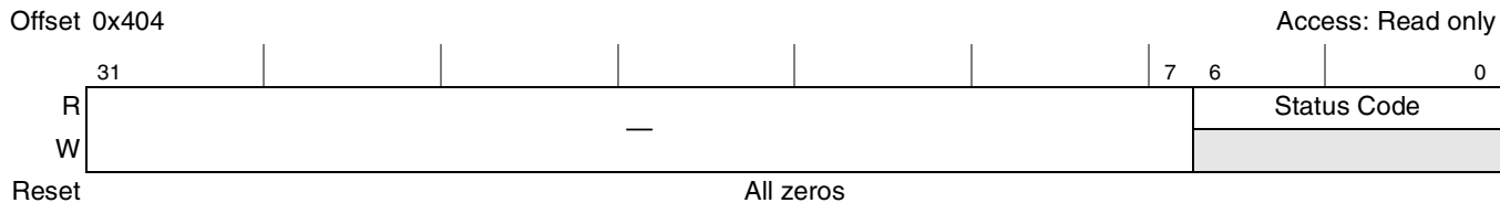
Figure 17-114. PCI Express LTSSM State Status Register (PEX_LTSSM_STAT)
