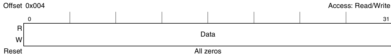
Figure 17-3. PCI Express Configuration Data Register (PEX_CONFIG_DATA)
