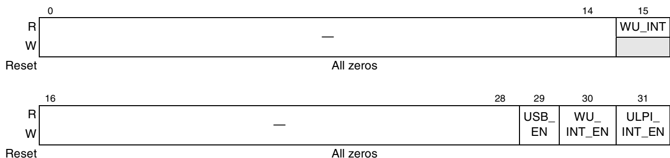
Figure 21-33. USB General-Purpose Register (CONTROL)
