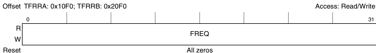
Figure 9-11. Timer Frequency Reporting Registers (TFRRx)
