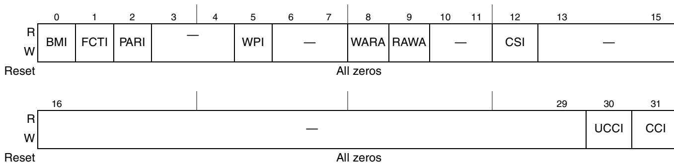
Figure 13-15. Transfer Error Interrupt Enable Register (LTEIR)
