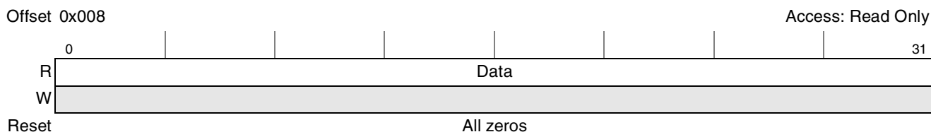
Figure 16-5. PCI INT_ACK Register
