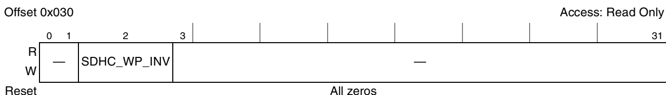
Figure 23-8. General Configuration Register (GENCFGR)
