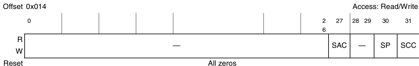
Figure 17-6. PCI Express Configuration Register (PEX_CONFIG)
