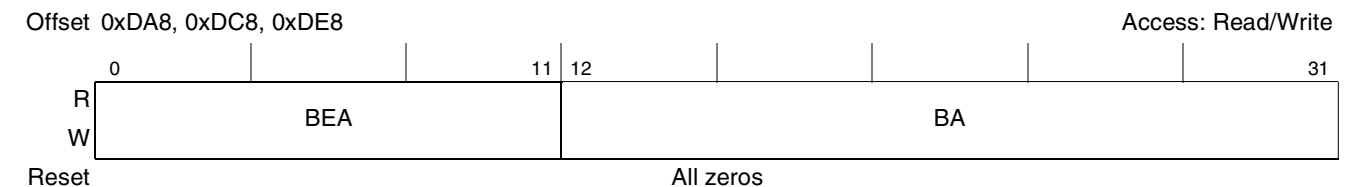
Figure 16-12. PCI Inbound Window Base Address Registers
