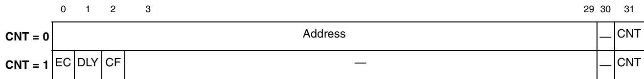
Figure 4-12. Config Address Fields
