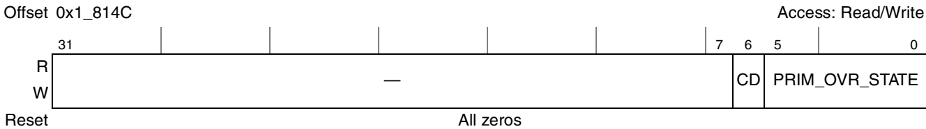
Figure 19-20. Link Layer Configuration Register1 (LinkCfg1)
