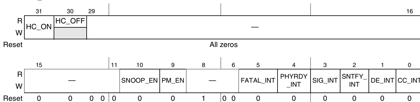
Figure 19-9. Host Control (HControl) Register
