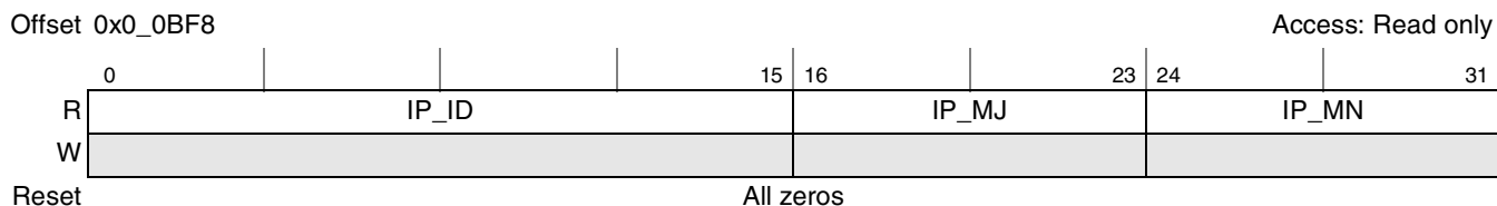
Figure 2-2. Local Access IP Block Revision Register 1 (LAIPBRR1)
