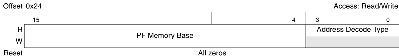
Figure 17-68. PCI Express Prefetchable Memory Base Register
