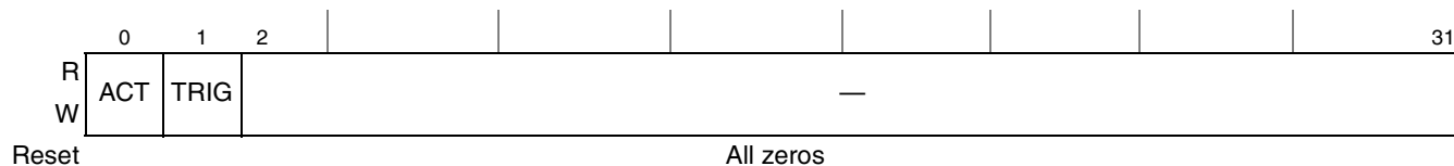
Figure 25-7. Watchpoint Monitor Status Register (WMSR)
