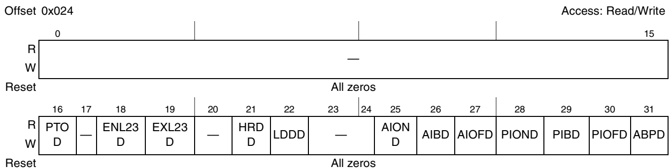
Figure 17-8. PCI Express PME and Message Disable Register (PEX_PME_MES_DISR)
