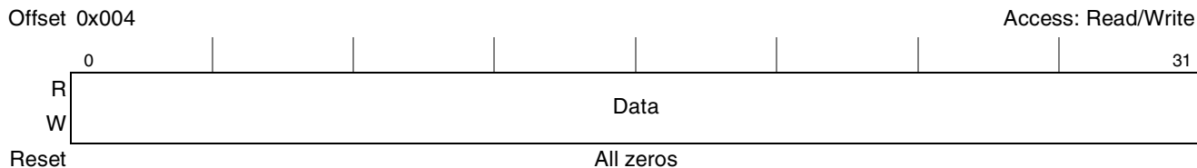
Figure 16-4. PCI CFG_DATA Register
