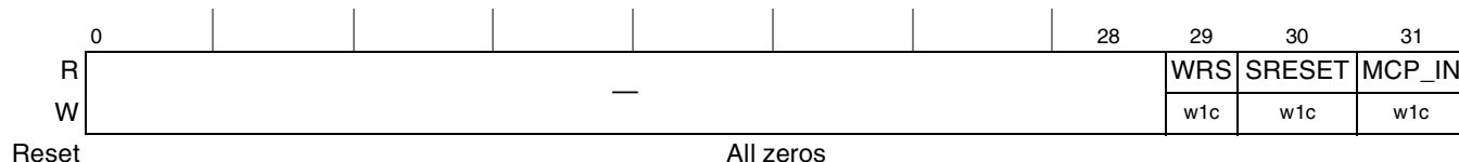
Figure 23-16. Machine Check Summary Register (MCPSUMR)
