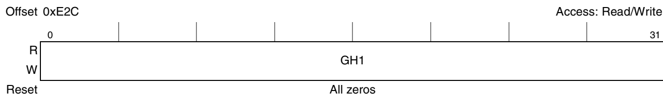
Figure 17-31. PCI Express Error Capture Register 1 (PEX_ERR_CAP_R1) External Source, Inbound Transaction
