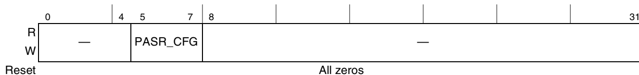
Figure 8-4. Chip Select Configuration Register 2 (CS n CONFIG 2)
