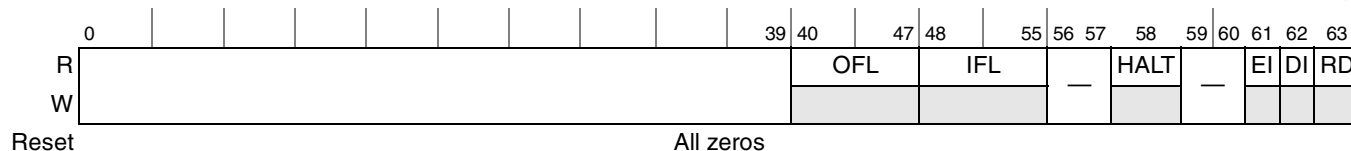
Figure 10-36. AFEU Status Register
