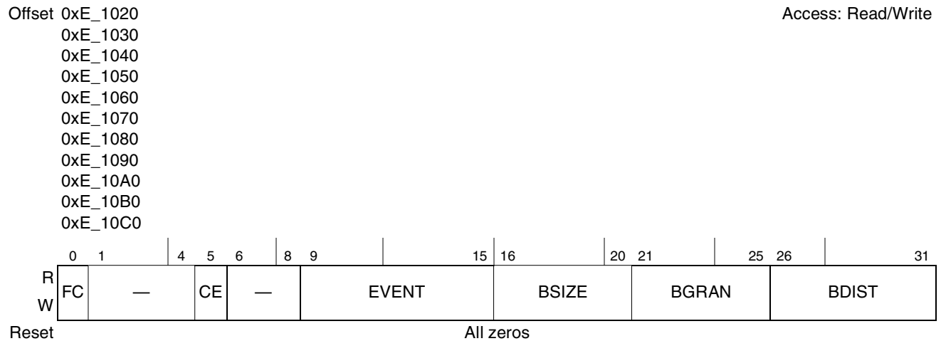
Figure 24-4. Performance Monitor Local Control A Registers (PMLCA1–PMLCA9)
