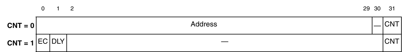
Figure 4-9. Config Address Fields
