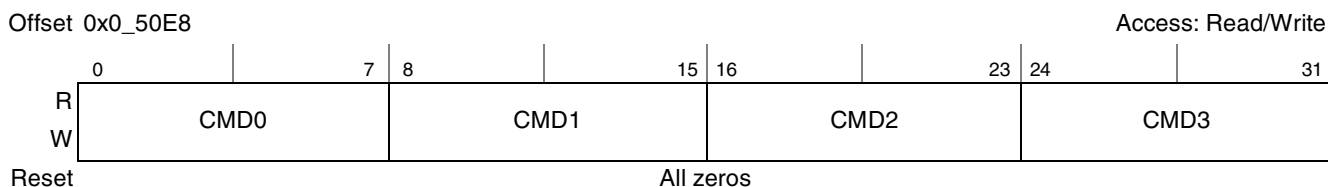
Figure 13-23. Flash Command Register
