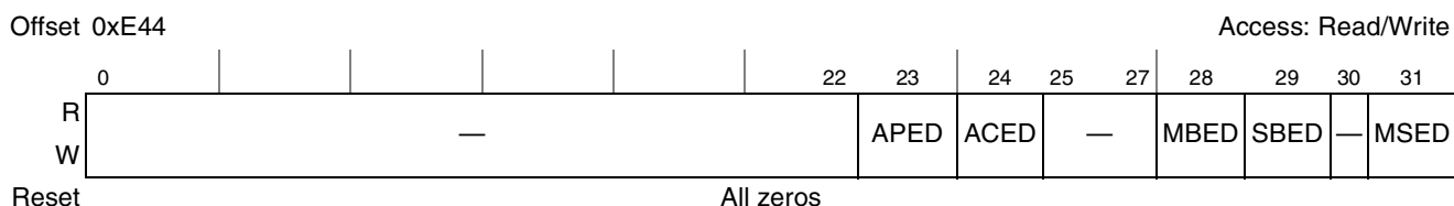
Figure 8-39. Memory Error Disable Register (ERR_DISABLE)
