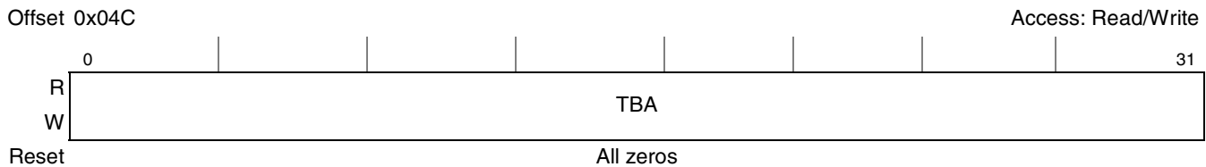
Figure 25-10. Trace Buffer Address Register (TBAR)
