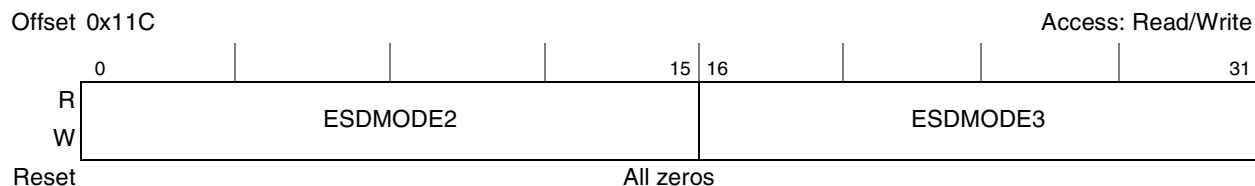
Figure 8-12. DDR SDRAM Mode 2 Configuration Register (DDR_SDRAM_MODE_2)
