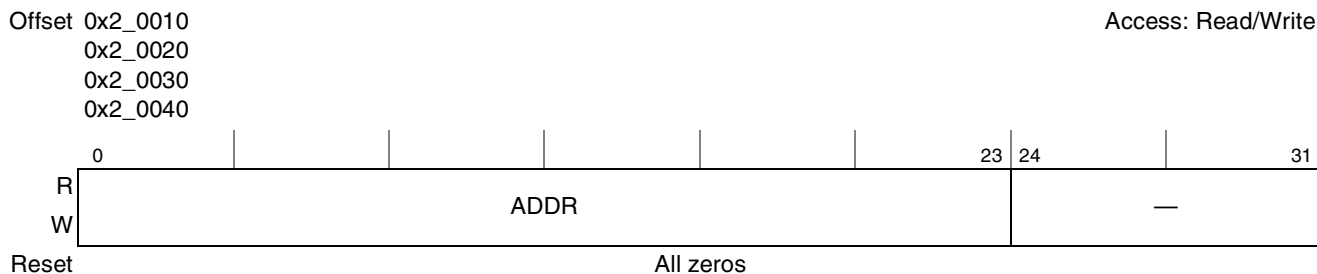
Figure 6-8. Cache External Write Address Registers (L2CEWAR n )
